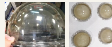
Before Improvement: Dome Cover Discoloration from Weather Exposure
