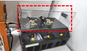
Prevention of exposed wiring in product live parts
